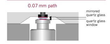
Figure 2: Sample drop squeezed between two quartz surfaces (0.07 mm path).
