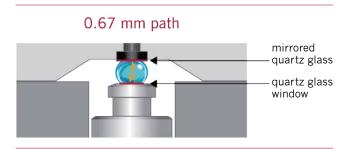
Figure 1: Sample drop squeezed between two quartz surfaces (0.67 mm path); light path indicated by orange arrows.
